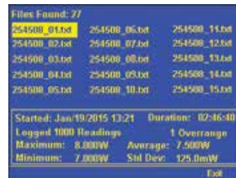
Data logs filed to USB Flash Drive. Can be viewed in StarLab or Excel.
