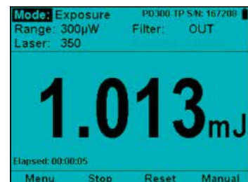
Exposure measurement (energy summing) with photodiode sensor.
