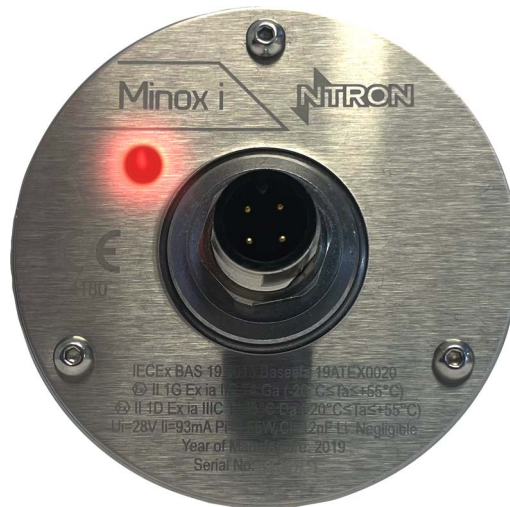
Figure 9. Minox-i indicator LED
