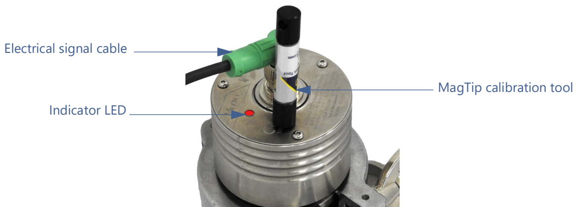
Figure 8. Minox-i with MagTip calibration tool
