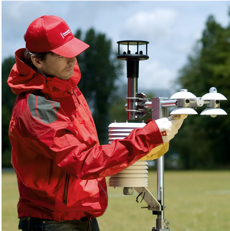
Figure 4.2.1 typical meteorological surface energy balance measurement system with HFP01SC installed under the soil.
