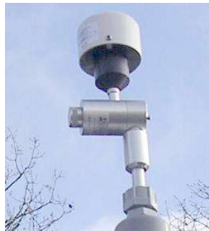
Figure 2-1 Sharp cut cyclone attached to intake
