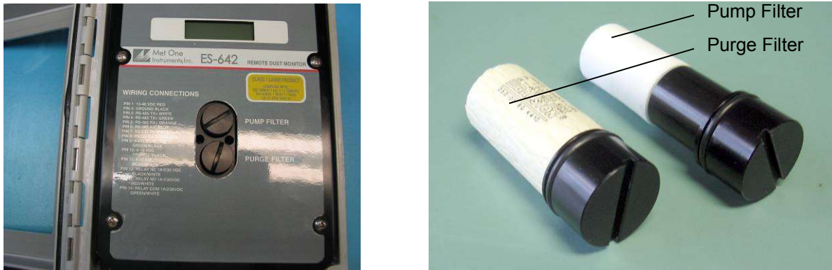
Figure 6-1 Pump Filter and Purge Filter Replacement
