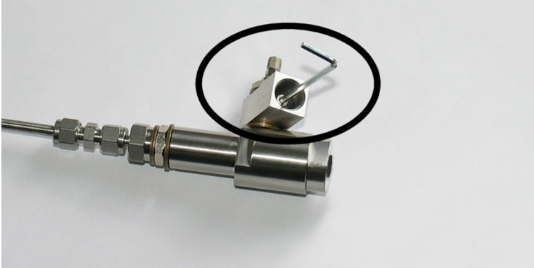
Figure 11 Removing the leak screw
